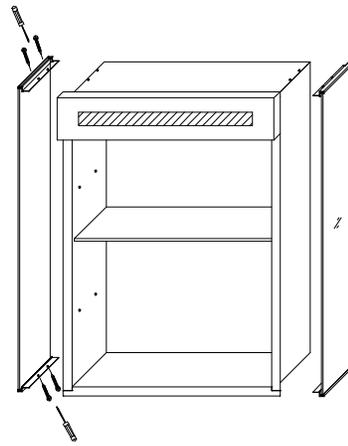
1. Remove the both of side mirror with a screwdriver.
