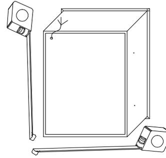
2. Measure the width and height of the back side of the cabinet.
