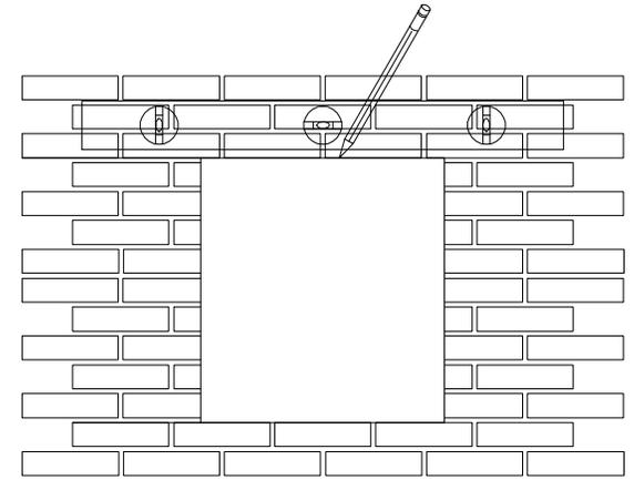
3. According to No.2, Draw a leveled rectangle on the wall with track level bar, that is about 1/5 inch larger than the cabinet recess in both width and height to make sure the fit not too tight. Make a hole that the depth is larger than 4.6 inch.
