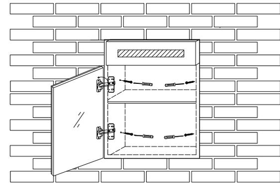
4. Insert the cabinet into the hole to test for size and position. If it seems to be where you want it. Install the screw on the left and right side of the cabinet.
